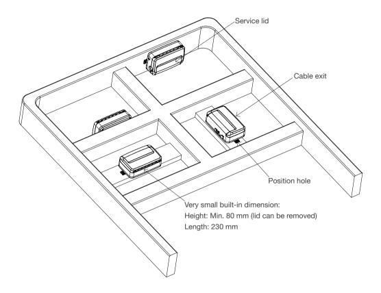
It is recommended to install JCB35T2 where it can drain water.
