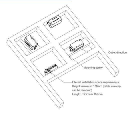
It is recommended that JCB35Q be installed in a position where it can drain water.
