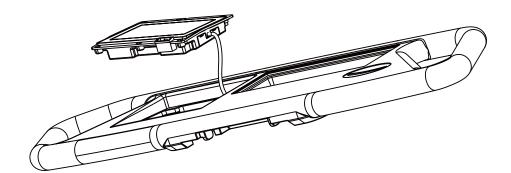
Step 5: Place the nurse's desk on the guardrail and secure it with 6 screws.
