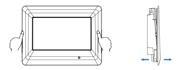
Step 2: Open the lower shell of dust cover for easy wiring insertion
