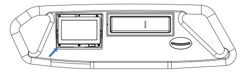
Screw's specification is 3.9\*16 disc head tip-tail screw
